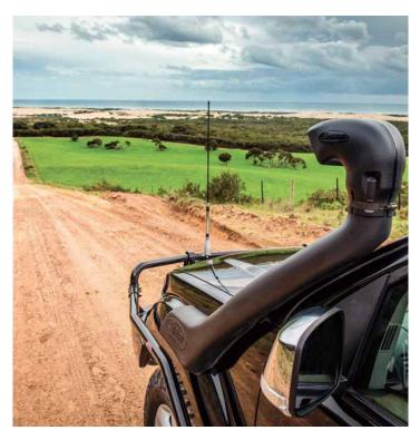
Created to protect 4WD engines from the hazards of dust and water ingestion commonly encountered in off road driving, Safari snorkels relocate your air intake point from the relatively low and vulnerable position under the bonnet to a higher and safer location, where a constant source of cool, clean, dry air is available.
