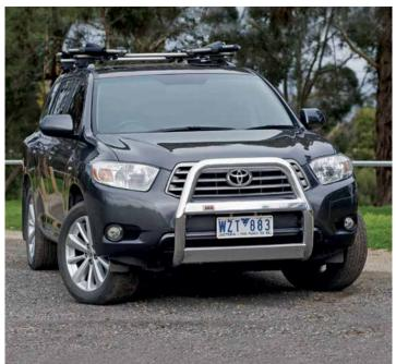
ARB manufactures both steel and aluminium nudge bars to suit a range of compact and medium sized SUVs, 2WD and 4WD vehicles. Like our range of bull bars, ARB's nudge bars are fully air bag compatible, provide increased frontal protection and add to the aesthetic appeal of your vehicle. Nudge bars also serve as an ideal platform for mounting accessories such as driving lights and CB antennas.
